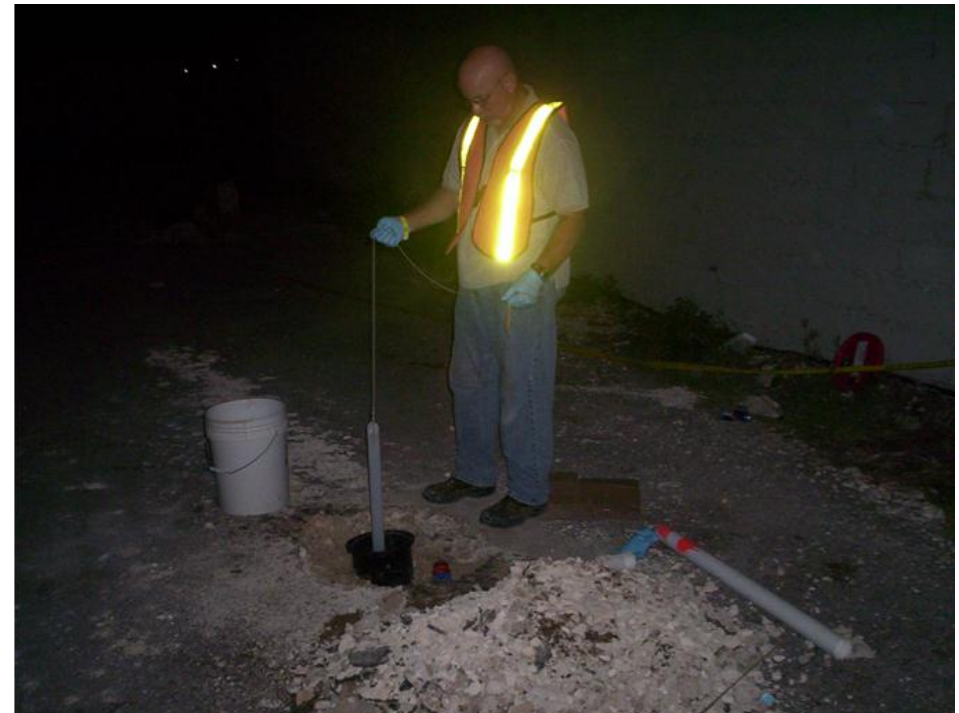
Ground water sampling at former ESSO Fuel Farm by Delta Environmental Consultant, USA
